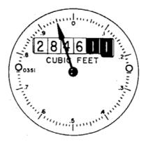
Some meters are circular with five or six dials. Read each dial clockwise, starting at the 100,000 dial. If a pointer is between two figures, read the lower number.
